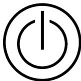
This button controls output power to connected load(s) and has dual functions: OFF and Bypass.
